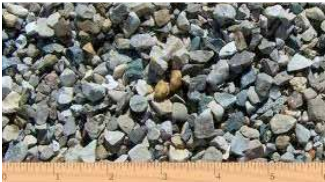
Figure 7: Examples of river gravel uncrushed and with crushed faces
