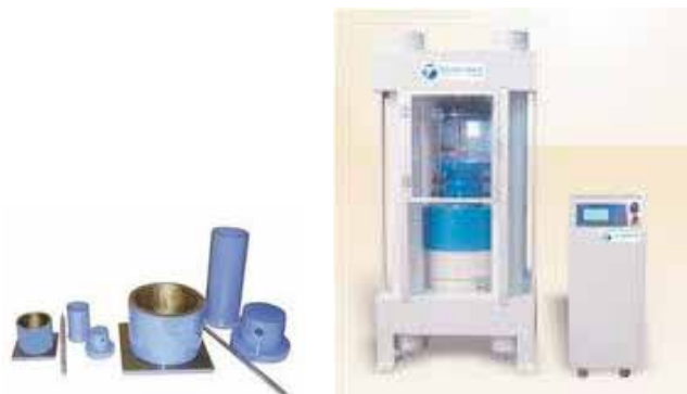
Figure 8: Wet/Dry strength test equipment and compression machine
