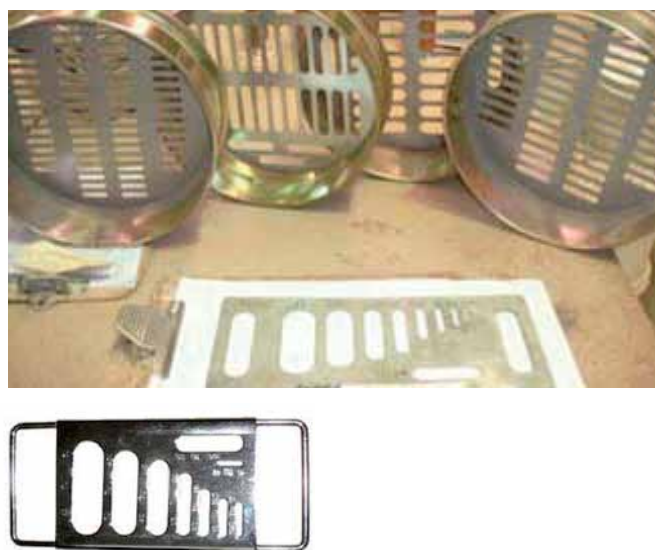
Figure 6: The Flakiness Index test gauge and Flakiness Index slotted sieves
