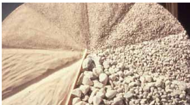
Figure 4: Combined aggregate and sand sample graded into its individual sizes
